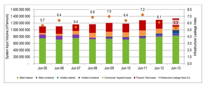
Per capita consumption peaked in 2009 at 325 \$\ell/c\rlor{d}\$ but has effectively remained constant over the past 8 to 9 years. The per capita consumption is based on the total system input volume and include industrial and commercial use. Ekurhuleni is the metro with the highest number of wet industries. The per capita consumption is slightly below the 2012/13 No Drop figure of 311 \$\ell/c\rlor{d}\$.
