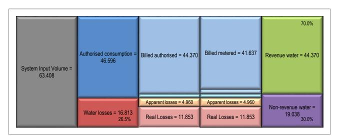
Water losses and NRW have been increasing consistently from 2005 to 2012, with a considerable reduction in non-revenue water realised in 2013. The drop in NRW and water losses is evident in Rustenburg and requires further investigation. The growth in system input volume has been exceptionally high in the past five years. Rustenburg and City of Tlokweng experienced a 9.82% and 5.77% five-year annualised growth respectively.
