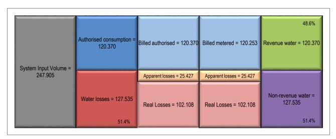
The NRW and water trends indicate consistent growth in system input volume, NRW and water losses over the past 9 years. Urgent attention must be given to the implementation of WCWDM as the water demand already exceeds the supply in large parts of the province.
