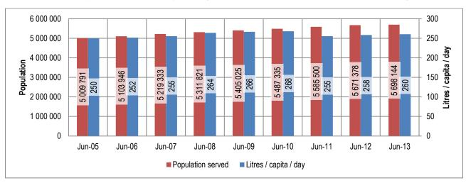
KwaZulu Natal has managed the maintain system input, leakage levels and per capita consumption in the past 5 to 6 years. With the looming / imposed water restrictions in the province, there is significant scope for improvement in reporting levels, data accuracy and a reduction of system input, NRW and water losses in the province.
