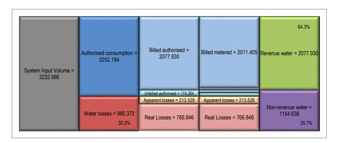
System input volume has been consistently increasing since 2006 but NRW has been improving since 2011 and water losses since 2009.
